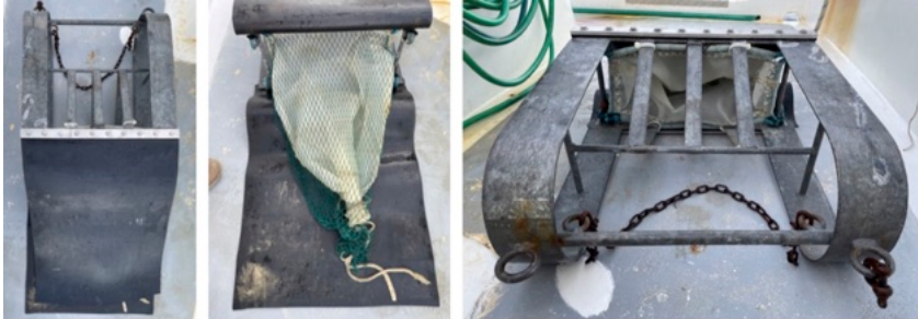
Figure 67: The Rauschert Dredge composed of a sledge-like metal frame drags the collecting megabenthic communities mesh bag (protected by rubber carpets) on the sea floor.
