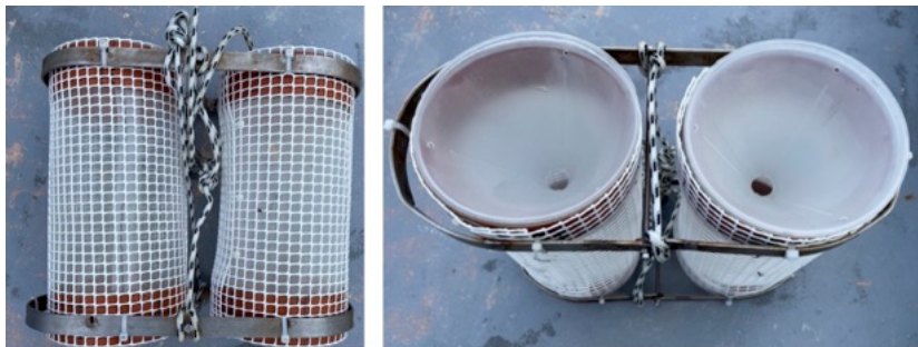
Figure 63: Baited amphipod trap composed of coarse plastic mesh for protection doubled by 500 \mu fine mesh. Both sides of the cylinder are equipped with a funnel to capture organisms into the trap
