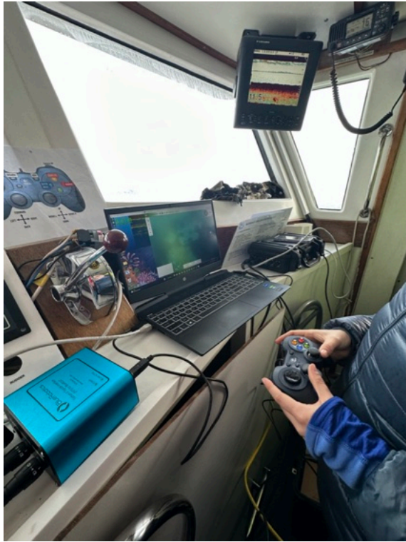
Figure 50: the Australis topside setup to control the BlueROV.
